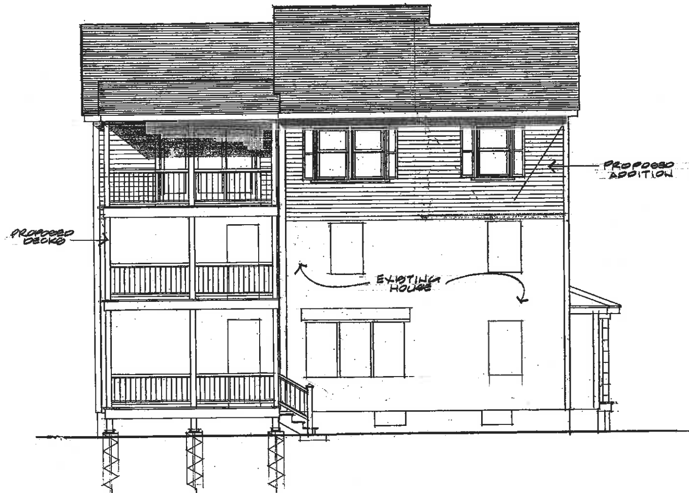
LEFT SIDE ELEVATION - BROOKS ST. 1/4" = 1'-0"
